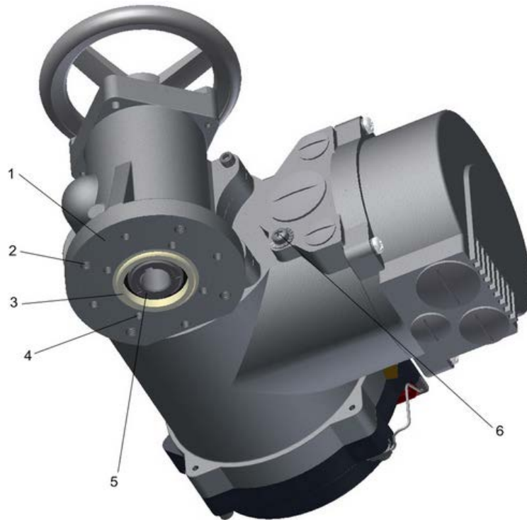
Figure 18: 1... mounting flange, 2... bore pattern G0/F10, 3... centring ring, 4... bore pattern F07, 5... shaft connection, 6... ground connection
